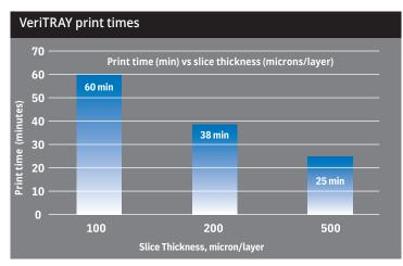
\* Data derived from printing VeriTRAY on Asiga Max 385 with a horizontal orientation and an object height of 3cm.
